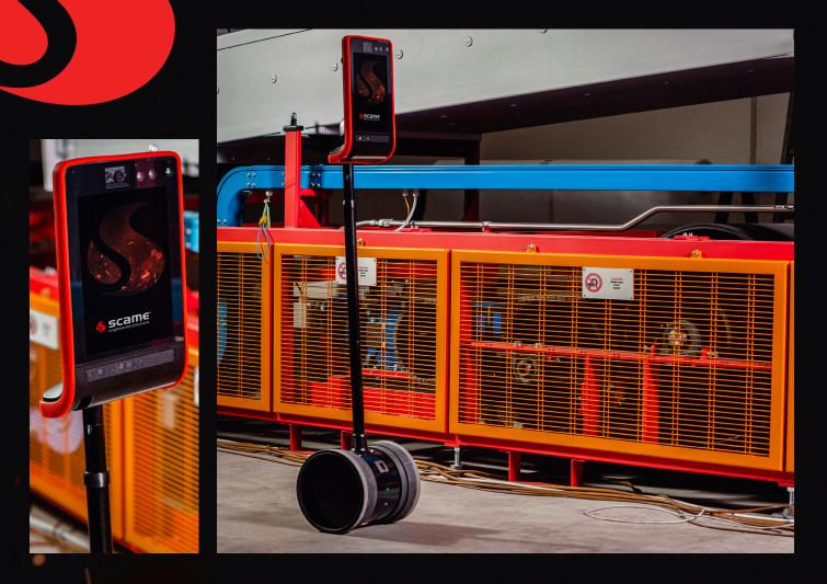
ScameBot is a remote communication robot with autonomous movement on two wheels wich allows to connect the technician with the customer's operator/maintenance worker - wherever it is located - and to provide DIAGNOSTICS and SUPPORT services as if it were physically on-site.
